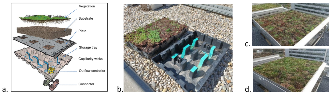
Figure 1. a) Scheme of the OASIS advanced green roof; b) photo of an unmounted tray; c) and d) photos in January 2023 of resp. Stromboli - 60 mm substrate and Monstro – 120 mm substrate. Adapted from Bertrand-Krajewski et al. (2024).
